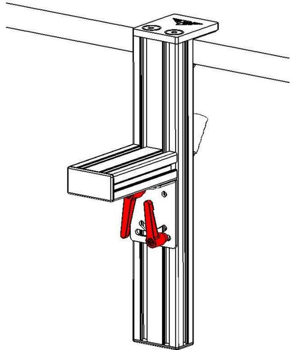
3. To tilt the second part of the Desk Mount clockwise, move the fixing handles.
