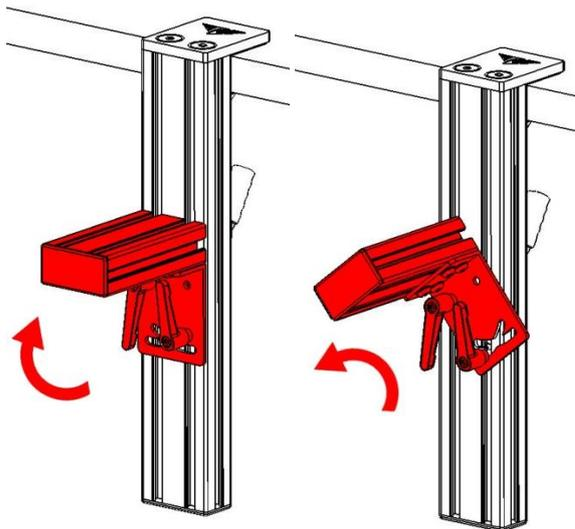
2. Tighten the fixing handles on the second part of the Desk Mount. \_\_\_\_\_
