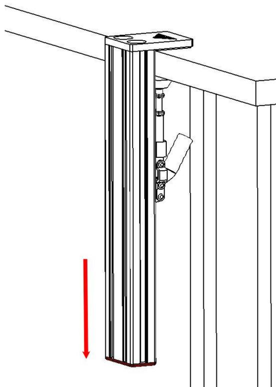
3. Install the Fixing handle with T-Nuts on the second part of the Desk Mount.
