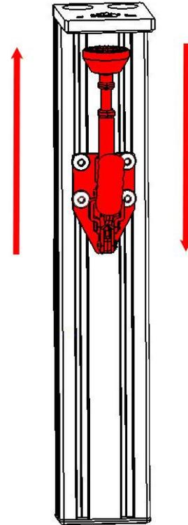
3. Tighten the screws after adjusting the clamp height.
