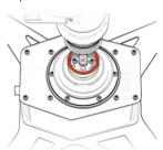
5. Adjust the position of the FC-35 Grip and tighten the indicated nut to the base
