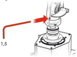
2. You can adjust the resistance by tightening or loosening the screw as shown in the figure
